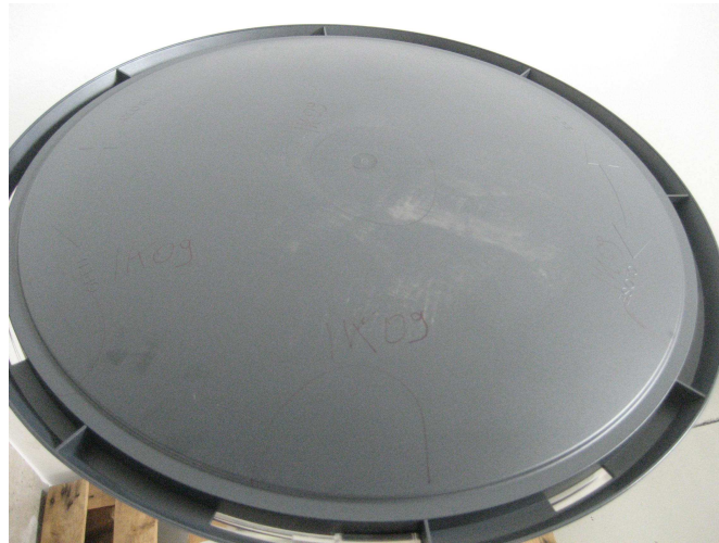
Photograph No. 4 Luminaire after IK09 (10J) Test.
