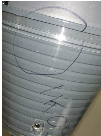
Photograph No. 6 Luminaire after IK09 (10J) Test.
