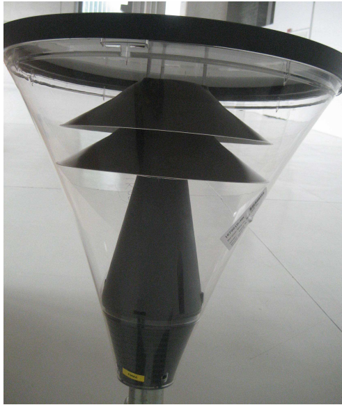
Photograph No. 3 Luminaire before IK05 (0,7J) Test.
