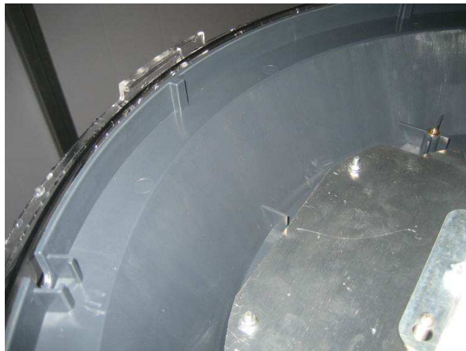
Photograph No. 12 Luminaire after IPX6 test (Pass no found water into luminaire)
