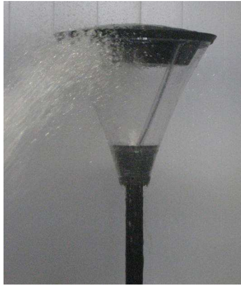
Photograph No. 7 Luminaire during IPX6 test
