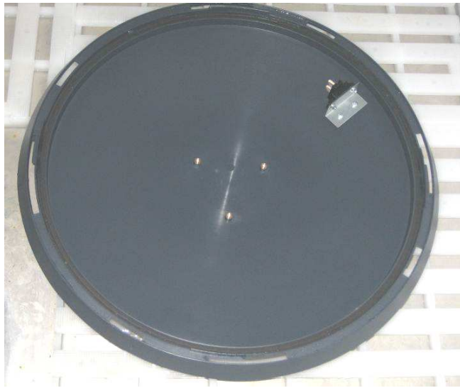
Photograph No. 10 Luminaire after IPX6 test (Pass no found water into luminaire)
