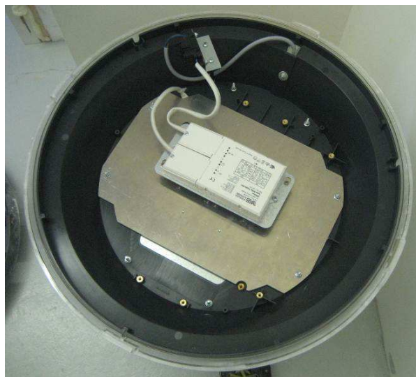
Photograph No. 4 Luminaire after IP6X Test.( Pass no dust into luminaire)
