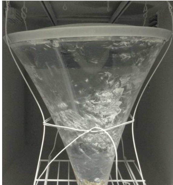
Photograph No. 3 Luminaire into test chamber after IP6X Test.
