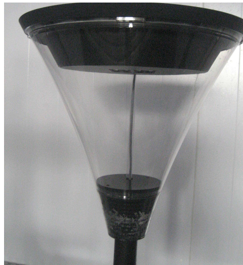
Photograph No. 8 Luminaire after IPX6 test (Pass no found water into luminaire)
